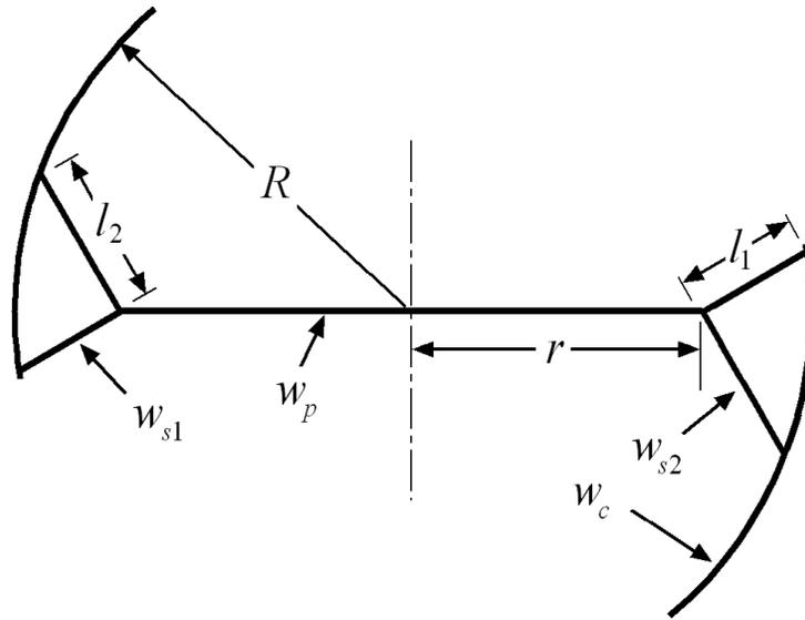
**Figure 1.** Plan view of the revolving elements of the 2-wing revolving door.
